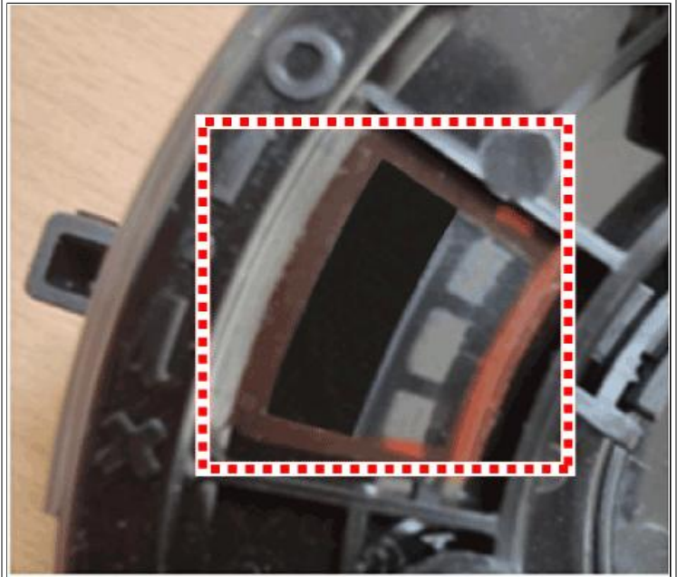
White cable is not visible through 10 O' Clock Neutral Check Window
